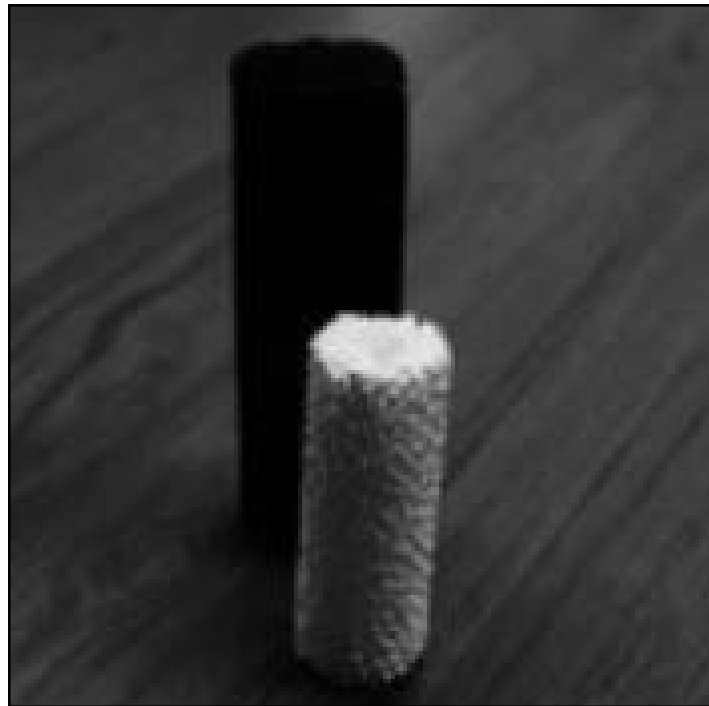
FOAM—Foam cylinders improve catalytic reactors in heat transfer by enhancing turbulence, mixing, and transport.
