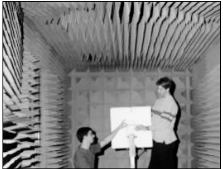
(Above)—Chris DeYoung, electrical engineering senior ( r. ), and Ben Fasenfest ( l. ) adjust a metal plate designed for positioning antennas in the anechoic chamber for on-site testing. (Below)—DeYoung sits at the control panel and makes adjustments in frequency and sensitivity for testing antennas.
