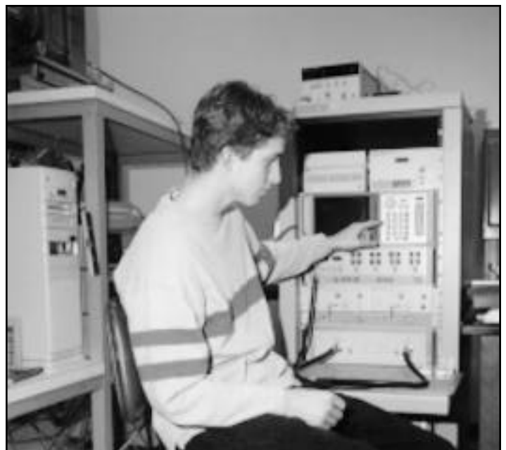
(Above)—Chris DeYoung, electrical engineering senior ( r. ), and Ben Fasenfest ( l. ) adjust a metal plate designed for positioning antennas in the anechoic chamber for on-site testing. (Below)—DeYoung sits at the control panel and makes adjustments in frequency and sensitivity for testing antennas.
