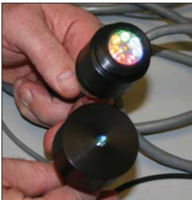
MINIATURIZATION —Discrete LEDs/photodetectors in the sensor (top) are shown with the chip-based sender (bottom) The sensor is less than 10 mm in diameter.
