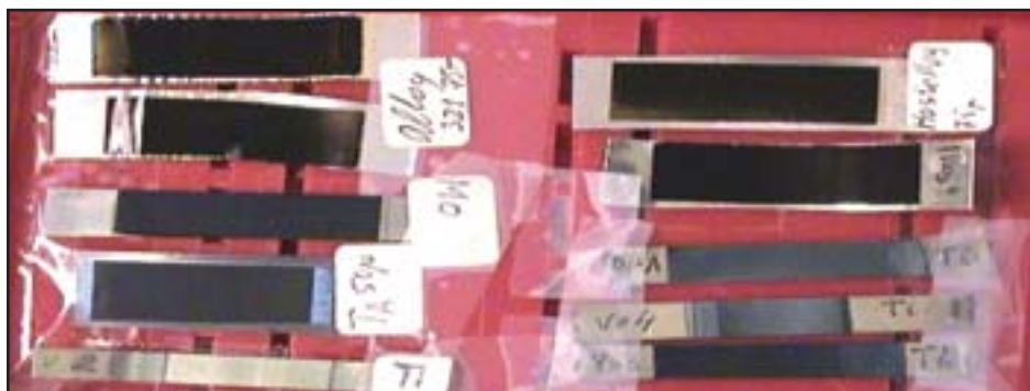
Figure 2. MCA Samples Fabricated Using Hastelloy, Alloy 321, Ta, Ti, and Mo Foils
