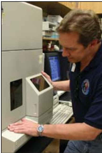
DNA —Dr. Mark Ott checks results in the genetic analyzer that sequences DNA. The equipment identifies genus and species of bacteria.
