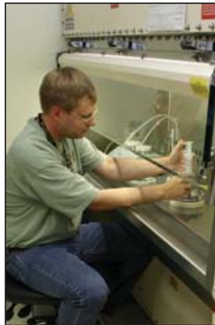
MICROGRAVITY —Dr. Don Tucker utilizes high aspect rotating vessels designed for modeling bacteria in a microgravity situation.
