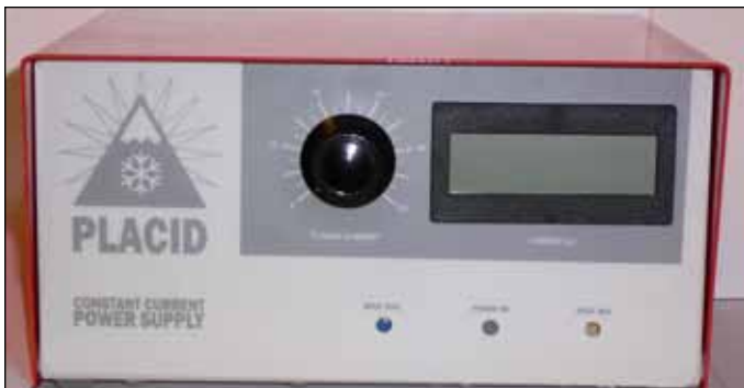
Figure 4. Magnetic Particle Brake Driver
