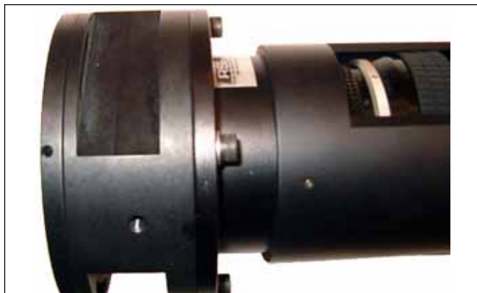
Figure 2. A micro-channel plate image intensifier with part of the coupling optics visible on the right. A cable (not shown) connects the intensifier to a power supply.
