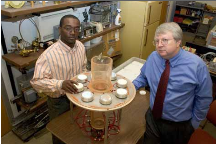
PAINT SAMPLES —Ashley Higgins ( l. ), master’s candidate in mechanical engineering, stands with Dr. D. Keith Hollingsworth ( r. ) with paint sample on metal coupons (disks) designed to test the effect of simulated martian dust on silicate paint, aluminum, and silver Teflon film.
