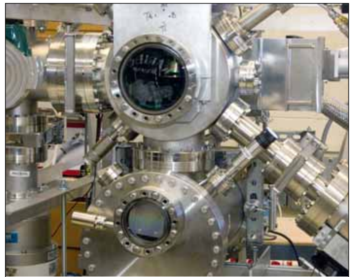
COATINGS—A multi-element coating reactor for hardcoating MCA structures in the Center for Advanced Materials. Such state-of-the-art equipment allows new technologies providing for the successful fabrication of micro-column arrays. Researchers are led by Dr. Abdelhak Bensaoula.
