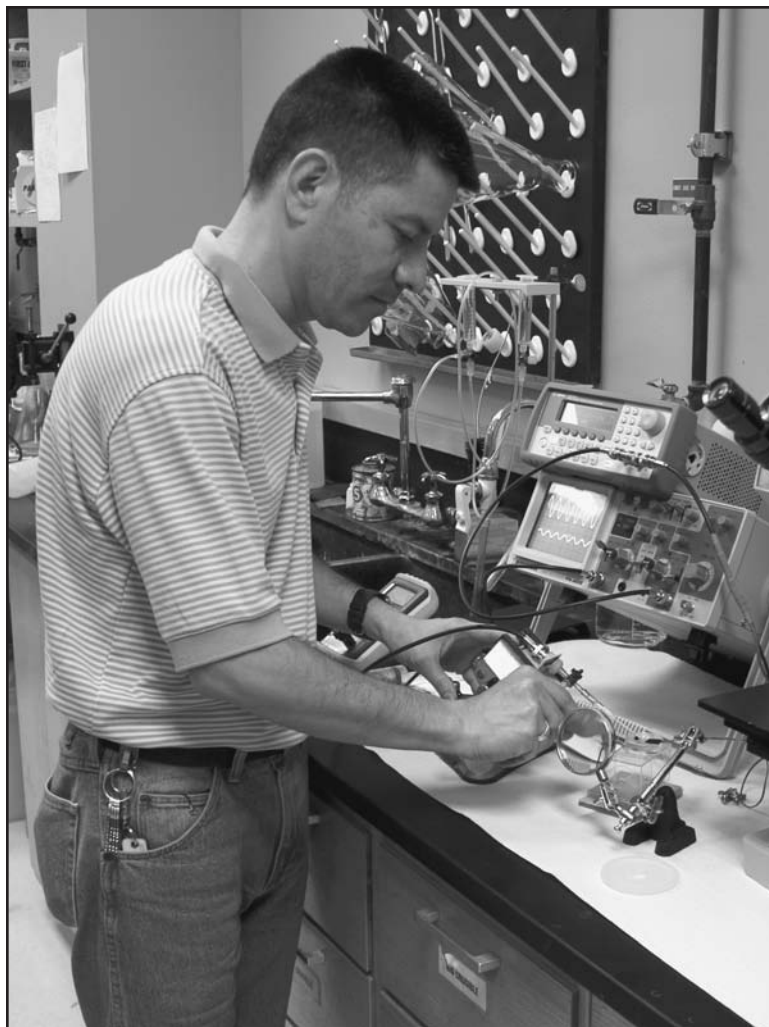
ELECTROMAGNETIC RESPONSES —Hans Infante, graduate student in physics, takes in-vitro measurements of electromagnetic responses of living cell suspensions utilizing superconducting quantum interference devices.
