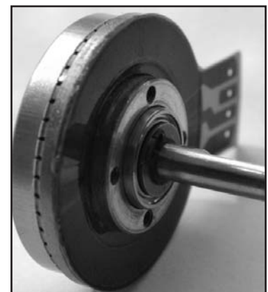
Figure 1. Piezo Systems Ultrasonic Motor (Shinsei USR30)
