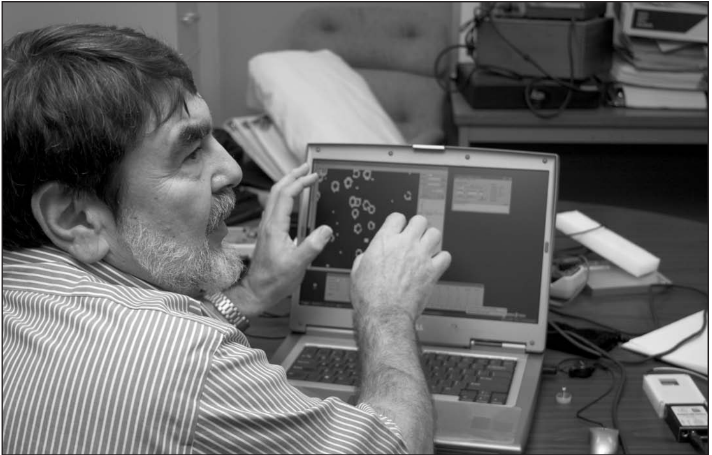
DOCIMETRY —Dr. Lawrence Pinsky, Physics Department chairman, shows a computer rendering captured from a newly designed docimeter which had been exposed to an alpha source. The circles on the display represent alpha particles hitting the detector.
